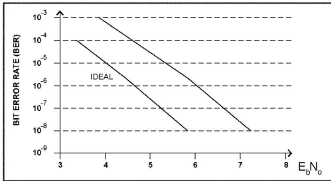
Figure 2-22. A typical example of the relationship of E_b/N_o to bit error rate (BER).
